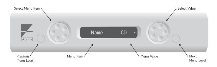
Use the left-hand knob to select which input (1 - 8) you wish to configure. Then press the right-hand button to enter the next menu level. The left-hand knob will select which setting you wish to configure for that input.
