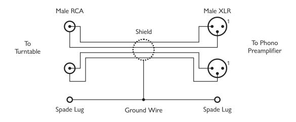
Please note that this configuration requires cabling that has a multiple of four conductors plus a shield. If there are eight or twelve conductors, they must be paralleled to create four composite conductors. Also, a short section of the cable jacket must be removed at each end of the custom cable to allow the connectors to be physically separated.
