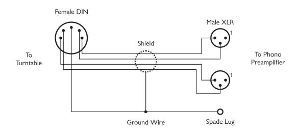
Remember that a section of the cable's outer jacket must be removed from each end of the custom cable. This provides a flexible section at the tonearm end, and allows the XLR connectors to be physically separated at the phono preamplifier end. In the event that a four conductor cable is not available, a pair of cables with at least two conductors each may be used as shown in the following diagram, with the DIN connector shown from the rear (solder) side:
