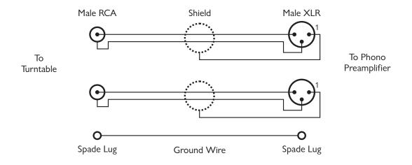
This configuration has two separate cables plus a ground wire, and requires balanced cabling with at least two conductors plus a shield. If the cabling has a third conductor (in addition to the shield), it should be connected to pin 1 of the XLR connector and left unconnected at the RCA end. If the cabling has four or more conductors, they should be paralleled to create two composite conductors.
