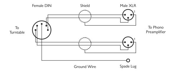
In this situation extra care must be taken to provide a flexible section to avoid interference with the turntable's suspension. If the cabling has three conductors (in addition to the shield), the third conductor should be connected to pin 1 of the XLR connectors and left unconnected at the tonearm end.
