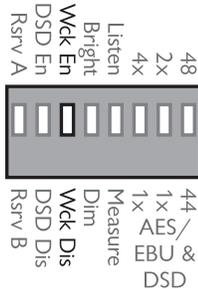
To enable the word clock outputs at the rate indicated on the front panel display, set the switch to the position labeled “Wck En”. Switch position “Wck Dis” will turn all the word clock outputs off.
