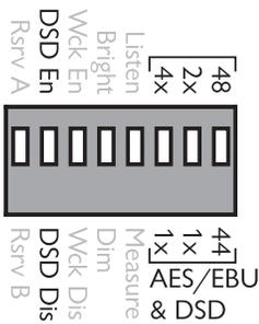
Three of the BNC output connectors can be configured to output digital audio data in the professional SDIF-2 or SDIF-3 DSD format. To enable the 3-wire DSD output set the switch to “DSD En”.
