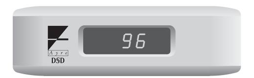
When your computer is powered on, the QB-9<sup>DSD</sup> will also enter the "Operate" mode. The display will indicate "---" to show it is ready to receive audio data. As the music file begins to play, the display will indicate the sample rate in kHz (e.g., "96"). When the music file stops, the display will revert to "---". Turning the computer off will also place the QB-9<sup>DSD</sup> back in "Standby" mode.
