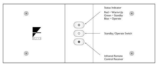
Should the AC line voltage drop below 80% of normal (brown-out), the unit will revert to "Warm-Up" mode and the indicator light will glow red. After the voltage returns to normal, the initial warm-up cycle will begin again.
